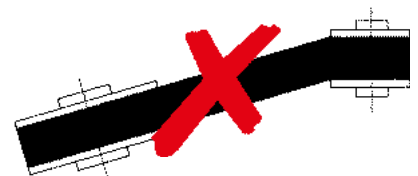
Horizontal angle deviation of the shafts
