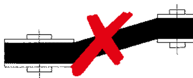
Axial misalignment of pulleys
